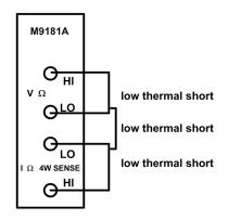
2 Now Perform the calibration process (see "Calibration Process" on page 16). Enter the calibration value of 0.00 for the calibration value (because the source is 0 V).
