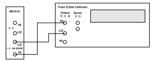
2 Apply the input signal shown in the "Input" column of the table. Enter the actual applied rms input voltage (see "Adjustments" on page 18).
