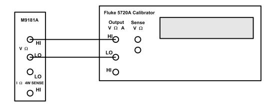
2 Apply the input signal shown in the "Input" column of the table. Enter the actual applied input voltage (for AC voltages enter RMS value) (see "Adjustments" on page 18).
