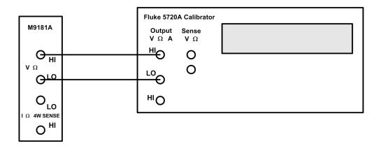
**3** Compare AC voltage measurement results from the M9181A DMM to the appropriate test limits shown in the table. Be certain to allow for appropriate source settling.
